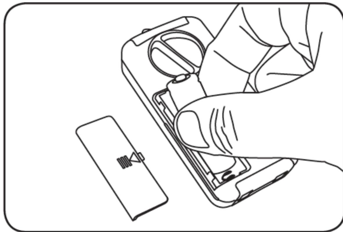
Remove the battery door from each of the light pendants by sliding in the direction of the arrow. Install an AA nickel metal hydride battery in each light pendant making sure that the negative end of the battery contacts the spring in the battery compartment and reinstall the battery door.
